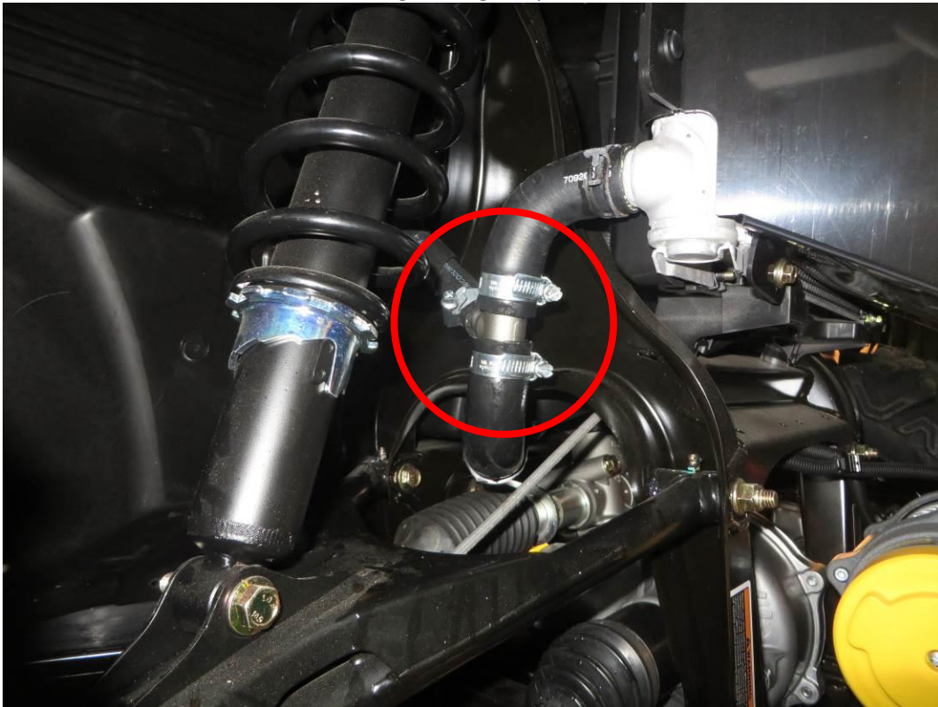
Cut the hose with the air vent to the correct length.
