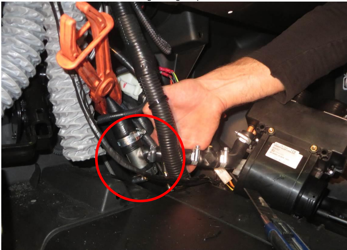
Connect the el, valve to the el.valve harness branch. DETAILED VIEW
