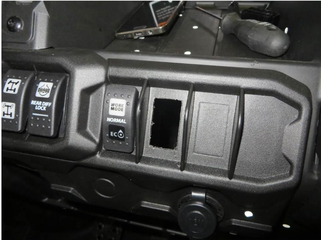
Connect the wiper/washer switch with the wiper/washer switch harness branch and press the switch into the dashboard.
