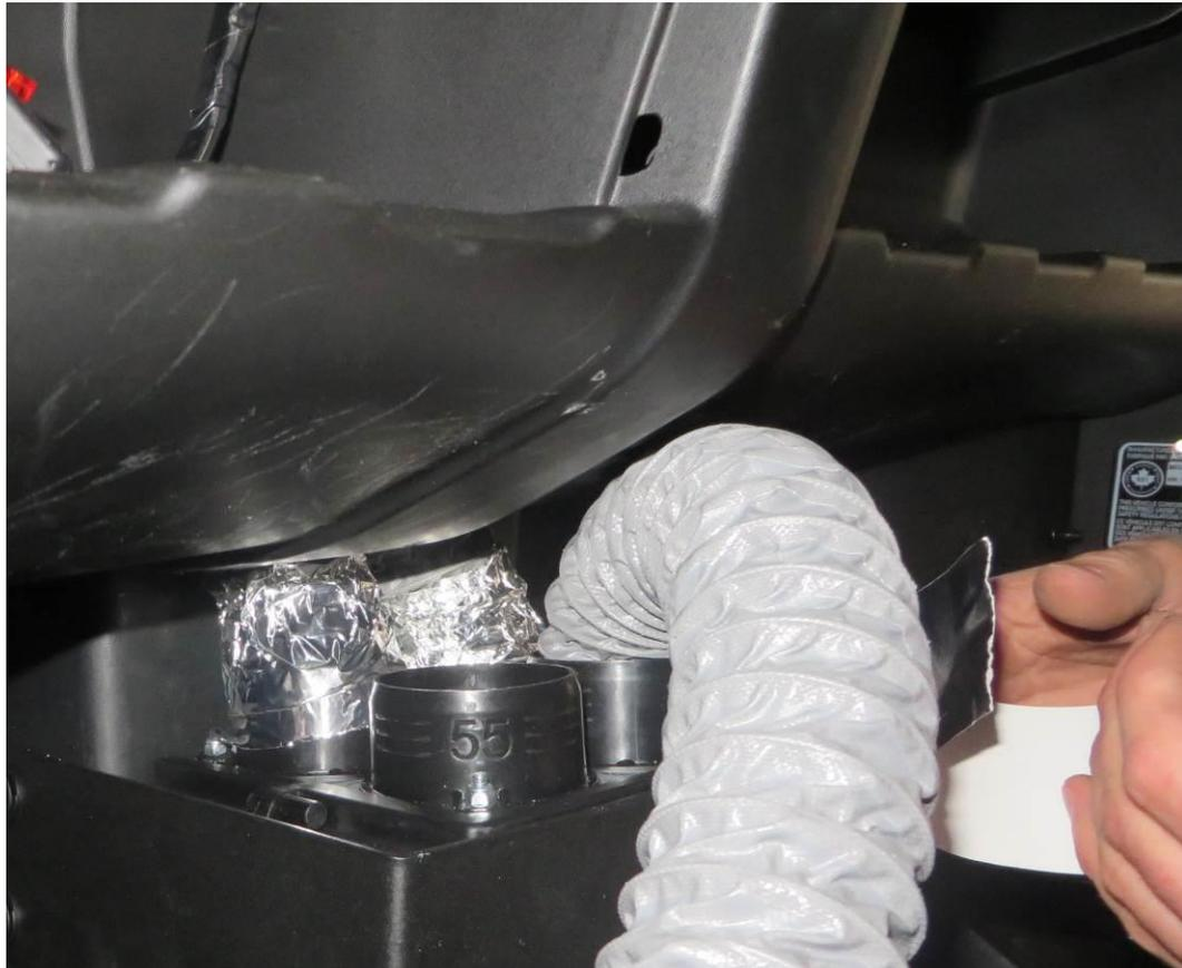
Prepare two shorter pieces of the hot air hose PVC to the rest of heater vents and fix by al. tape.
