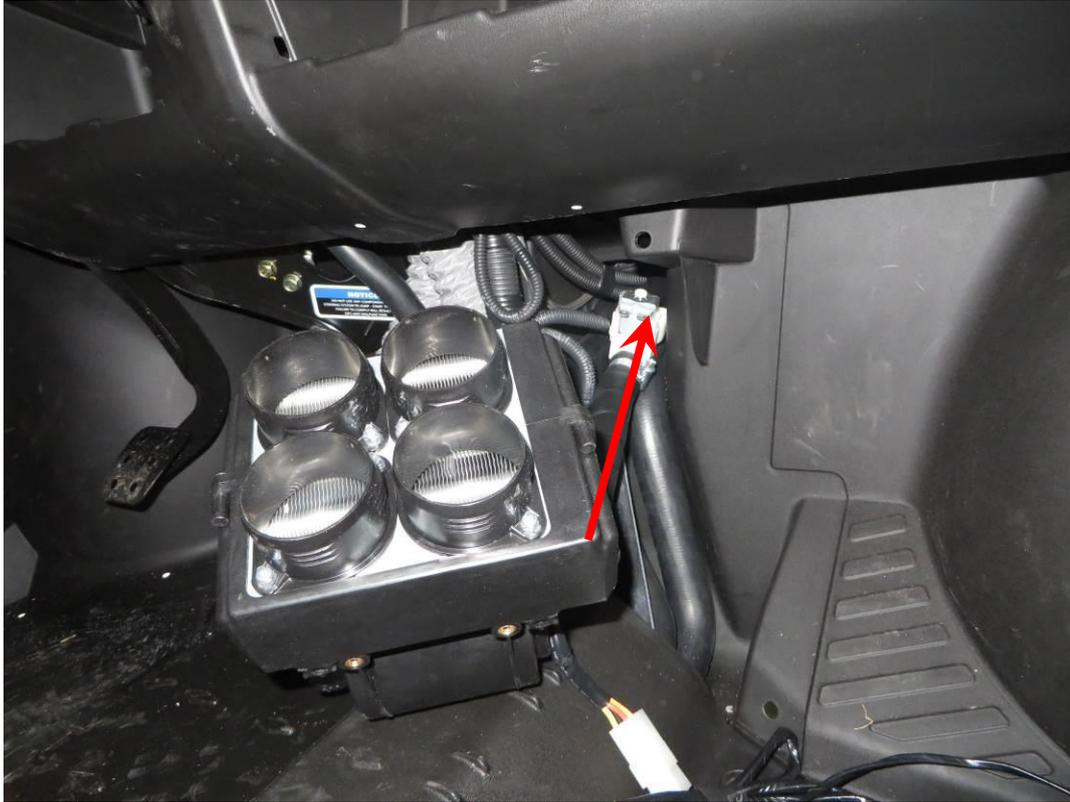
Cut the hot water hose and install the hot water pump, fix the hot water pump by tightening straps and tighten hard.
