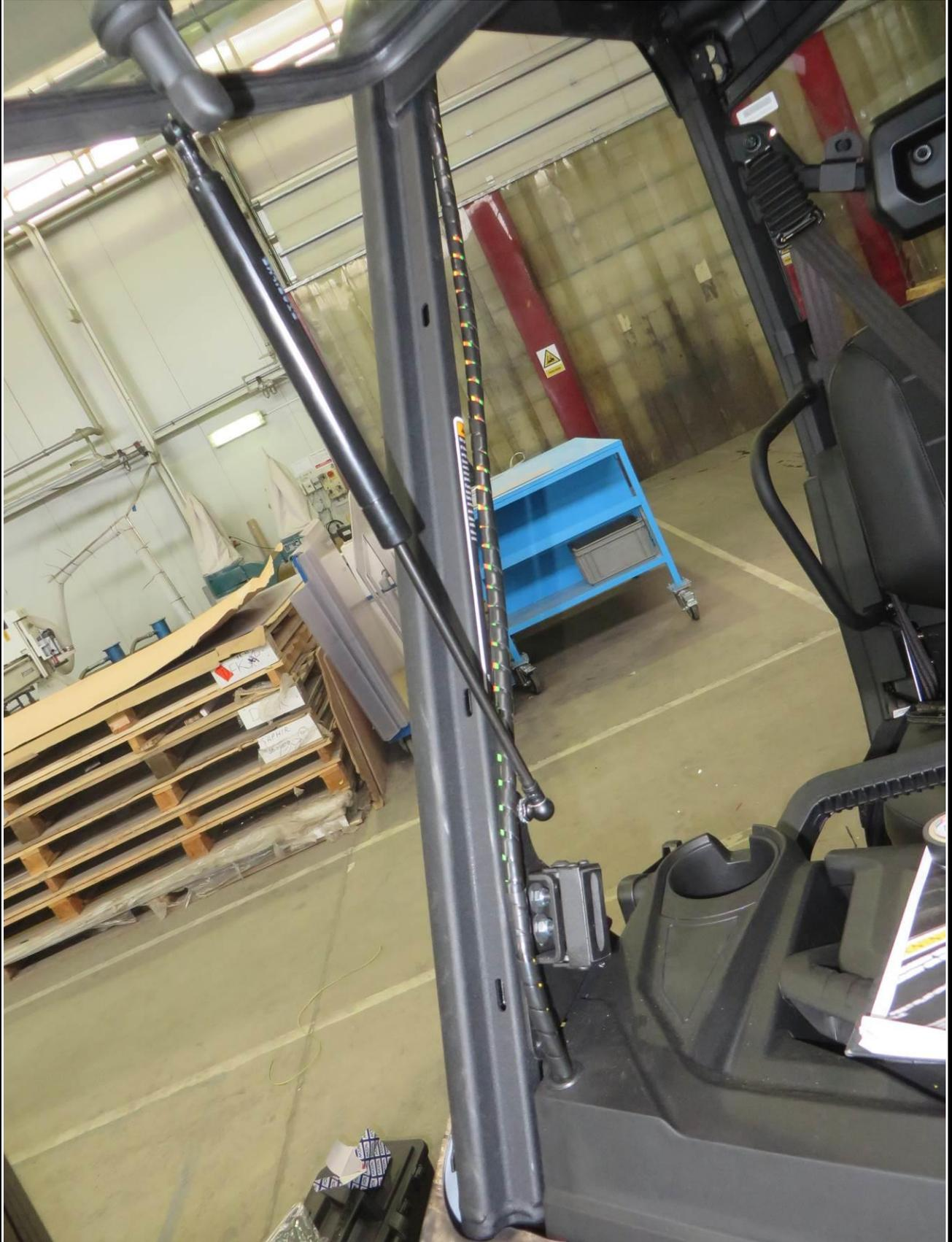
Install the harness cover ledge into the position and fix by included fixing assemblies. Lead the washer tube through the front glass and connect the tube to the washer jet.
