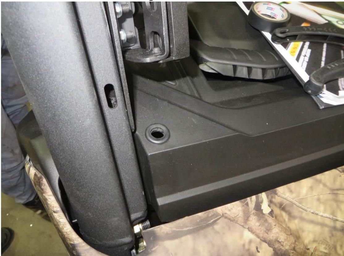
Lead the wiper motor harness branch with the washer tube around the UTV roller cage to the wiper motor.
