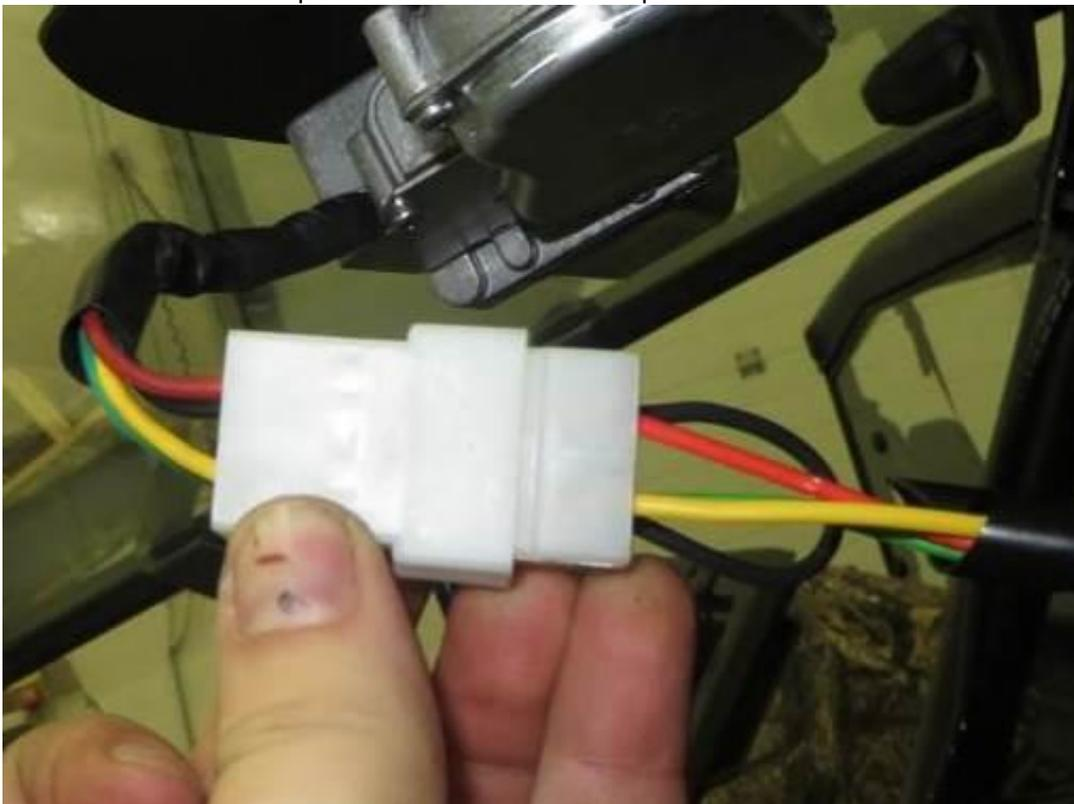
Connect the wiper washer harness to the UTV original electroinstallation.
