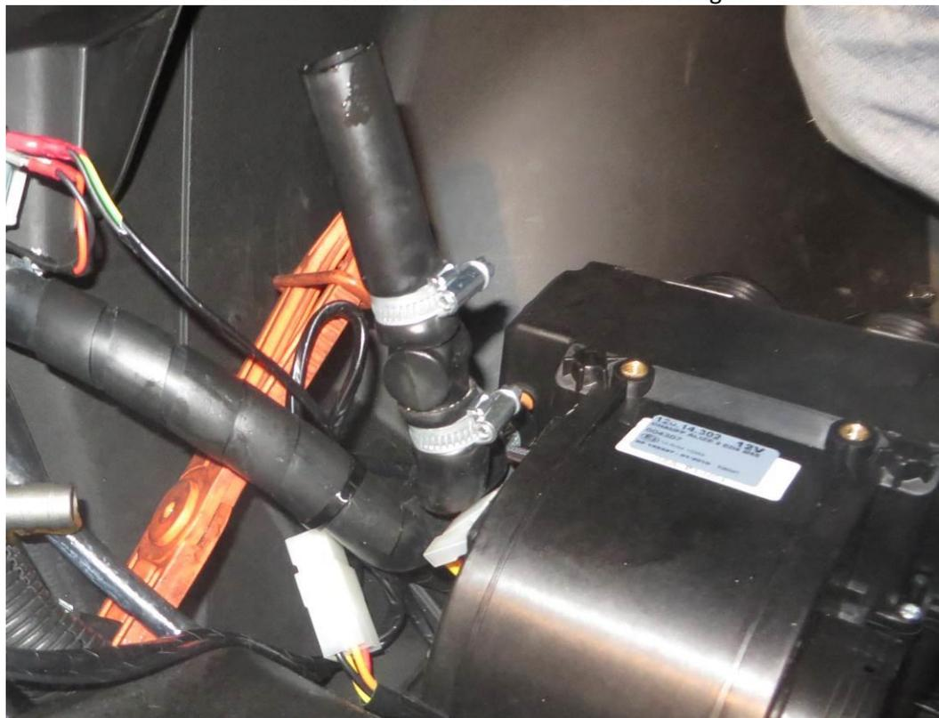
Secure the original cooling system cold water hose by clamps (not included), cut the hose and install included "Y" coupling into the hose. Connect the heater hose to the coupling and fix all ends by included tightening straps.
