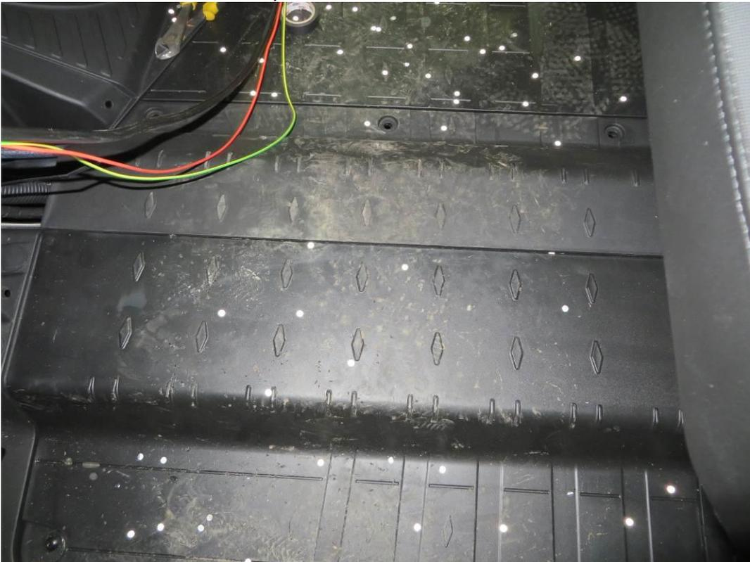
Lead the washer harness through the central tunnel and under the dashboard.
