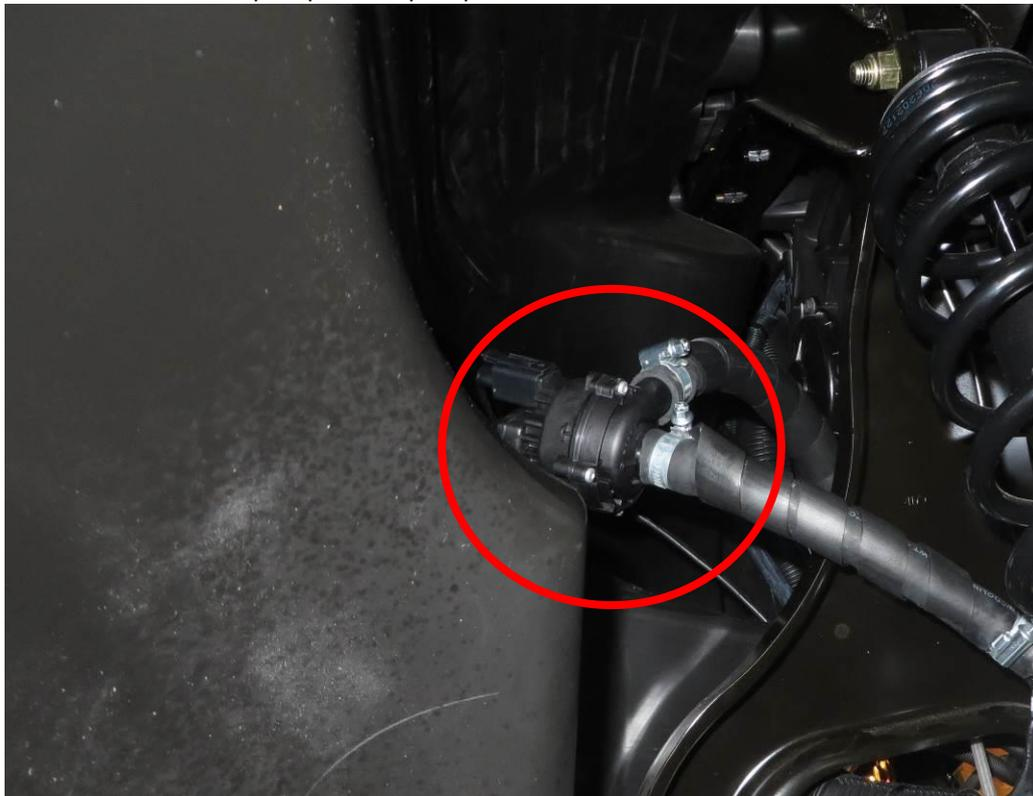
Secure the original cooling system hot water hose by clamps (not included), cut the hose and install included "Y" coupling into the hose. Connect the heater hose to the coupling and fix all ends by included tightening straps.
