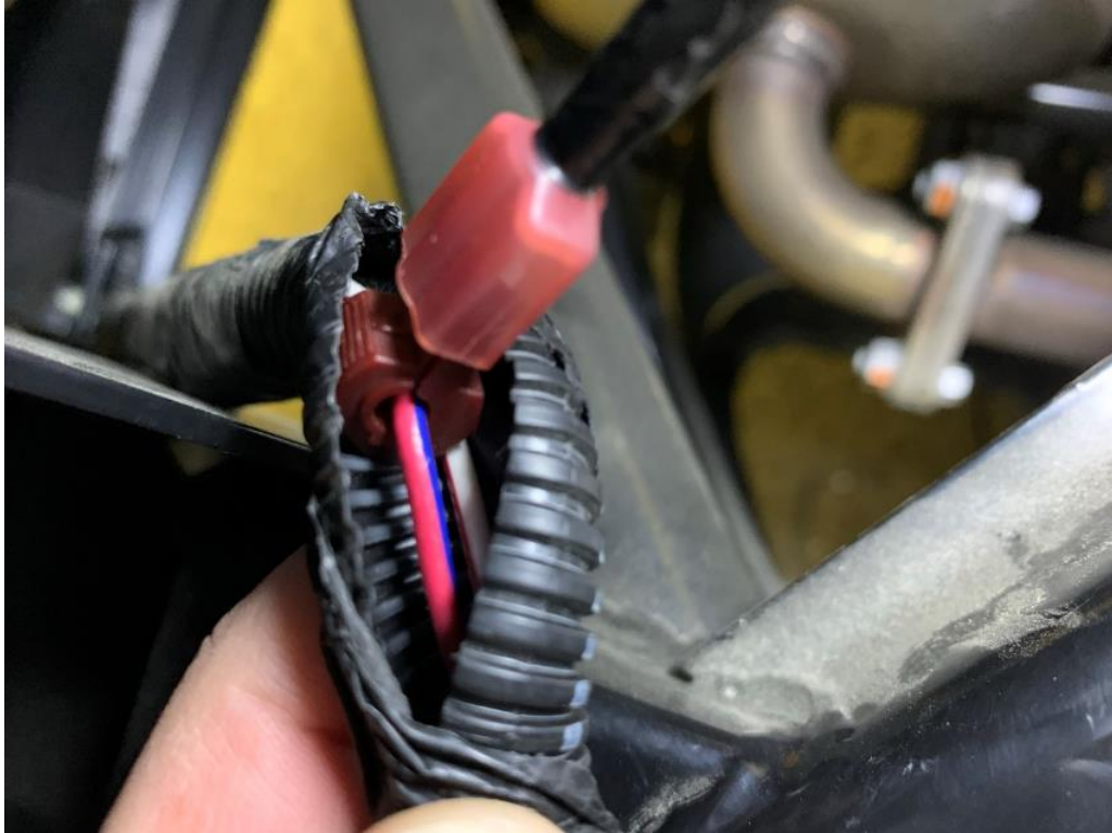
Connect the brake light harness black wire with the vehicle battery -12V.
