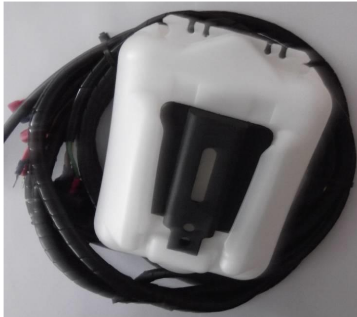
Harness and washer tank
