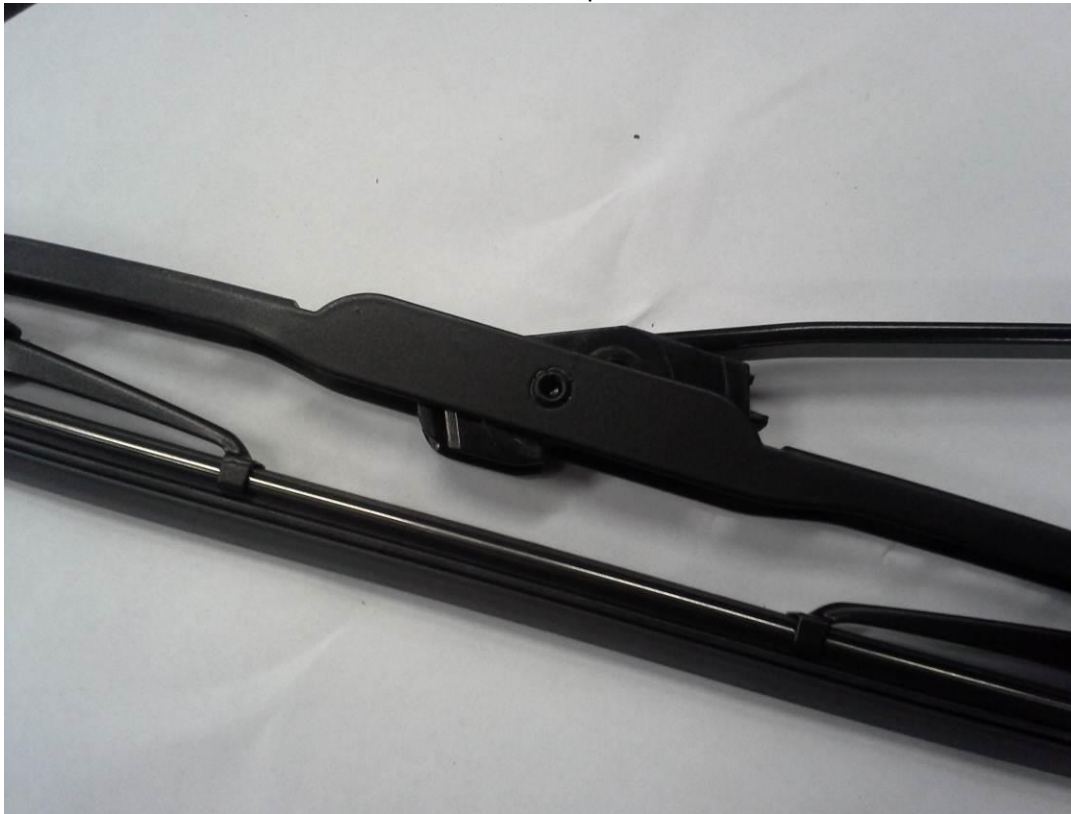
View onto installed wiper arm hook.
