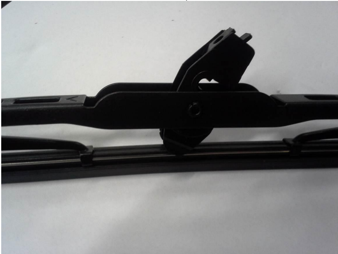
View onto the installed plastic holder.
