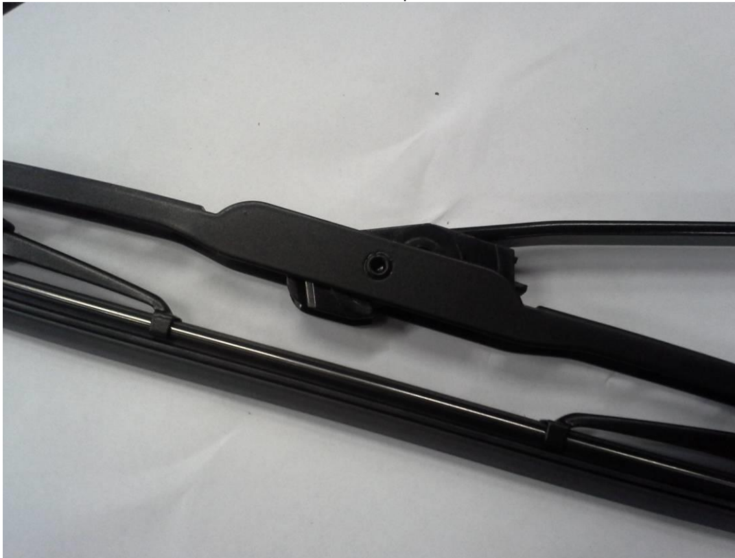
View onto installed wiper arm hook.
