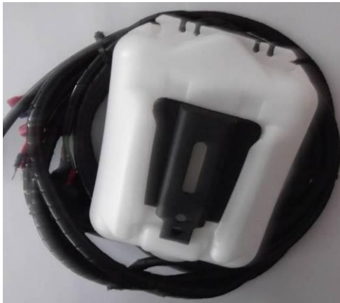
Harness and washer tank
