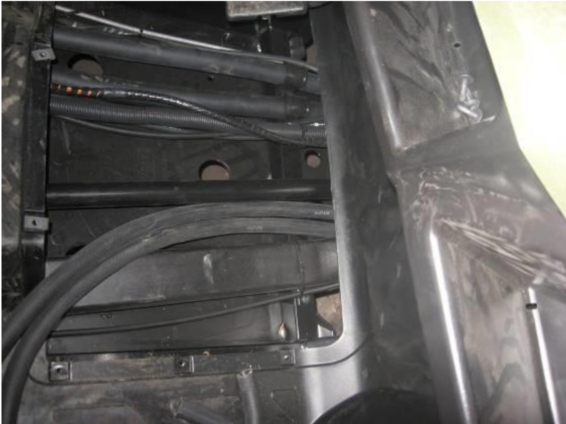
Water hoses in the floor tunnel.
