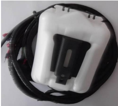
Harness and washer tank
