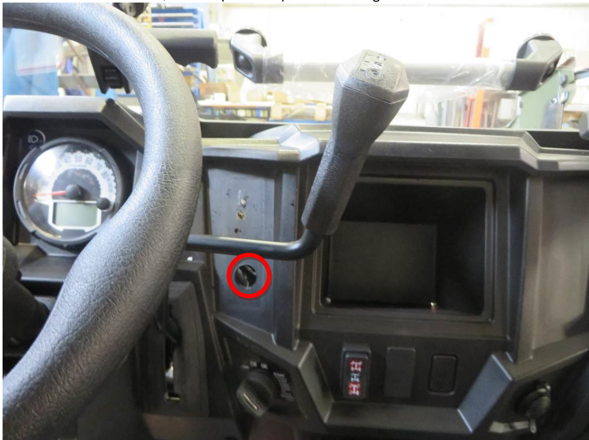
Drill hole \varnothing 21 mm (red circle) for electromagnetic vent switch.
