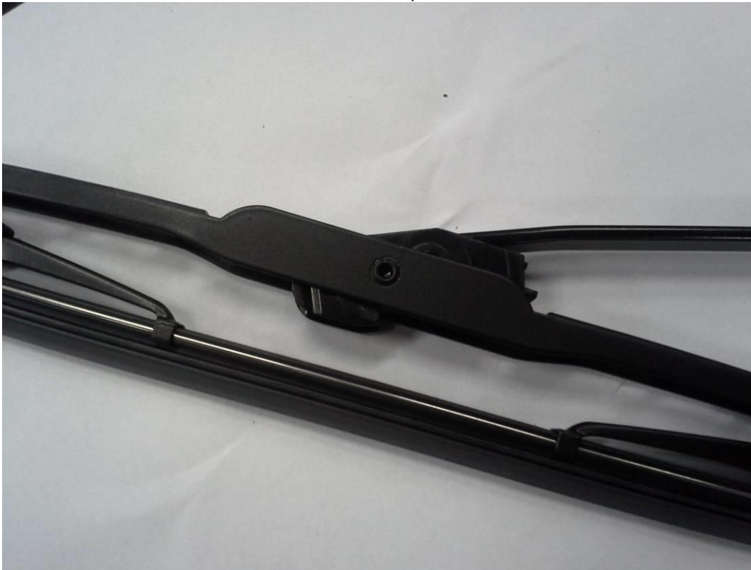
View onto installed wiper arm hook.
