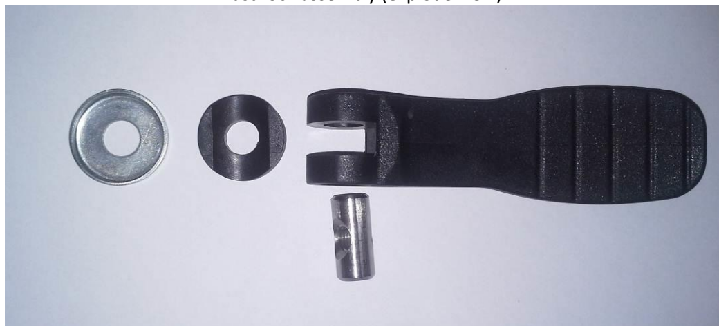
Fast-lock assembly (explode view).
