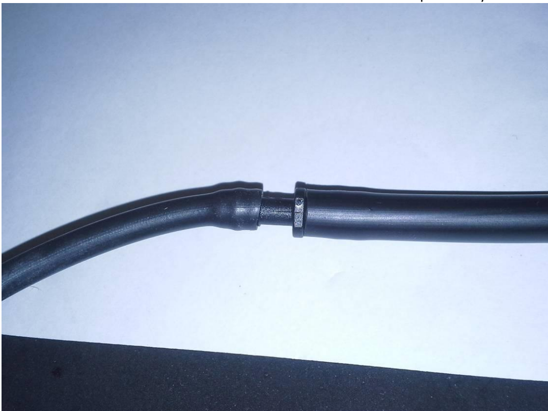
Connect the washer hose from the harness with the washer hose from wiper arm by included tube.
