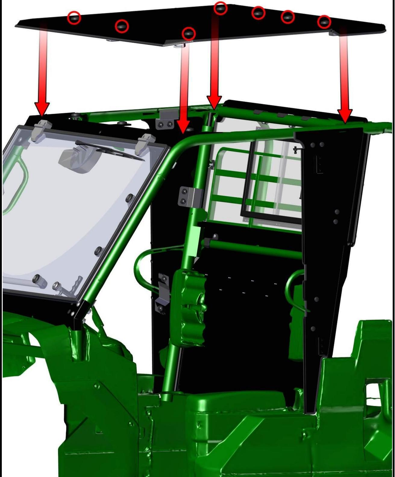
Turn the rear roof holder into the correct position and tighten.
