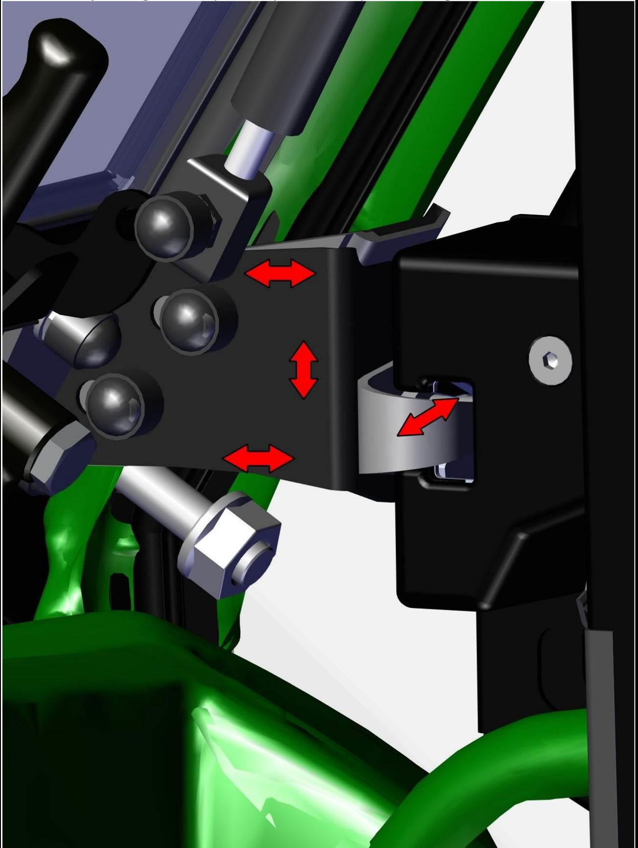
Install the gas spring pins into the gas spring holders in same orientation as on picture below.
