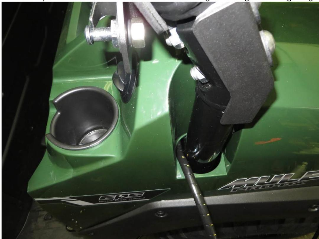
Lead the wiper/washer switch branch through the dashboard and connect the harness to the switch.
