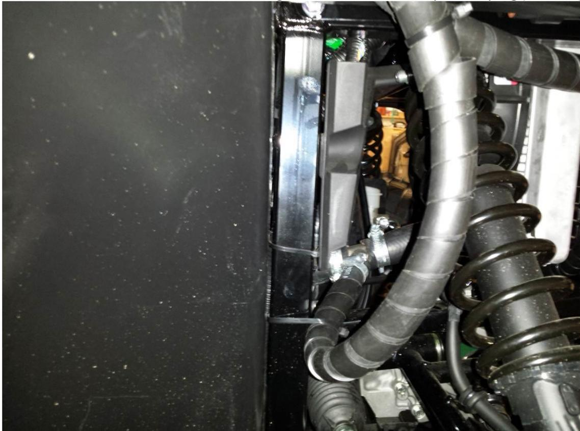
Lead the second hot water hose under the UTV floor to the engine.
