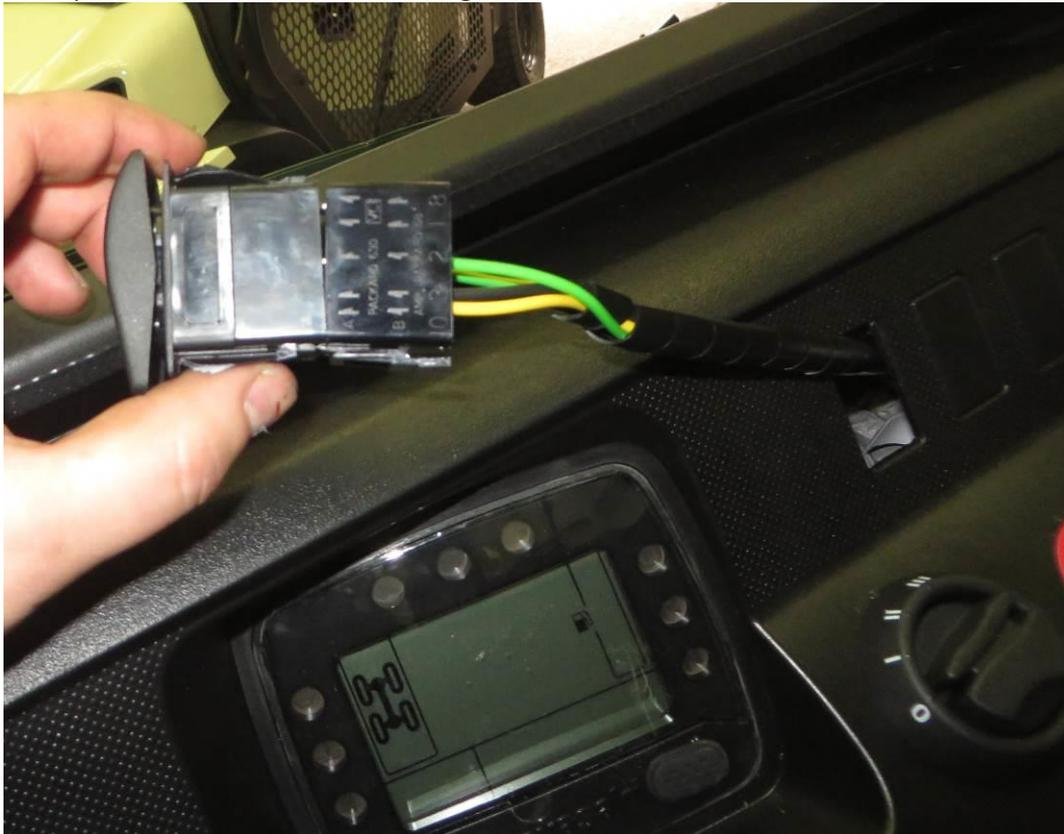
Press the switch into the dashboard. **INSTALL ALL PLASTIC COVERS BACK.**
