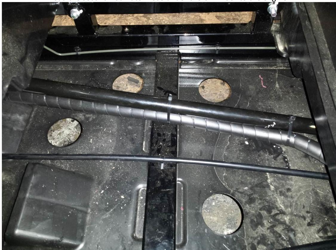
Connect hot water hose with the UTV's cooling circuit near the engine by "Y" coupling (included).
