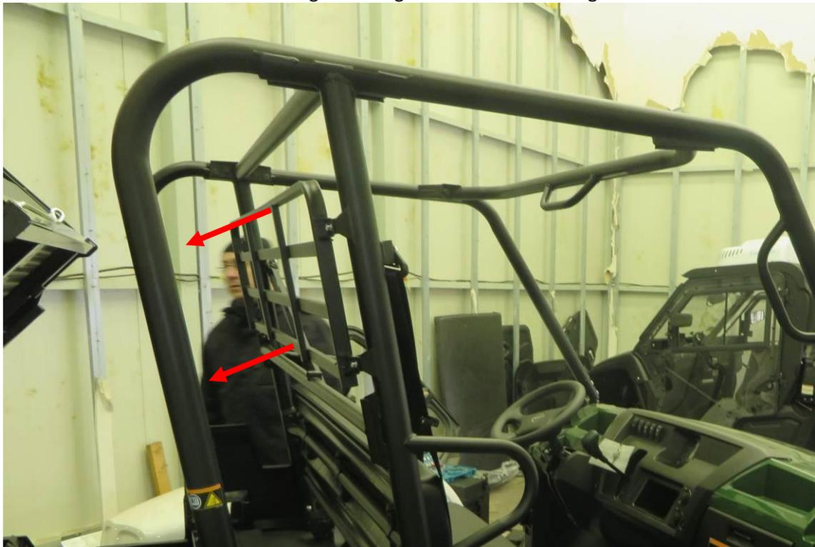
Loosen the rear bottom panel holders screws and place the rear bottom panel onto the UTV roller cage.
