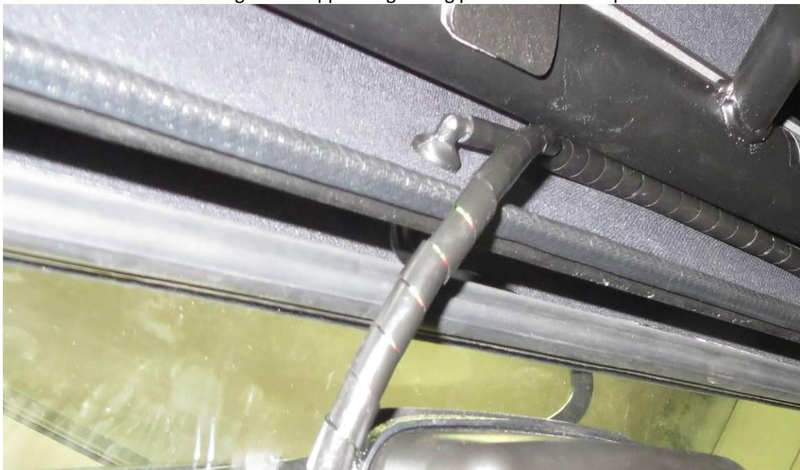
Connect the washer tube to the washer jet.
