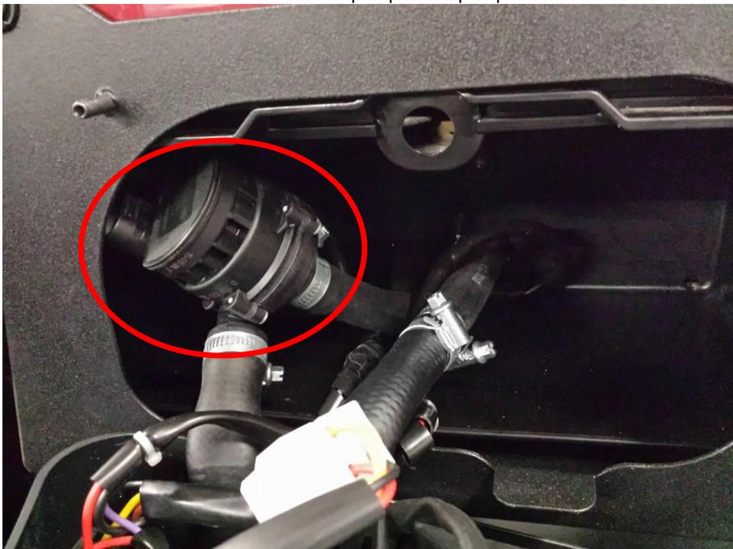
Install the heater holder to best position (heater assembly covers the glove box) and fix these with the UTV's body by included rubber rivets.
