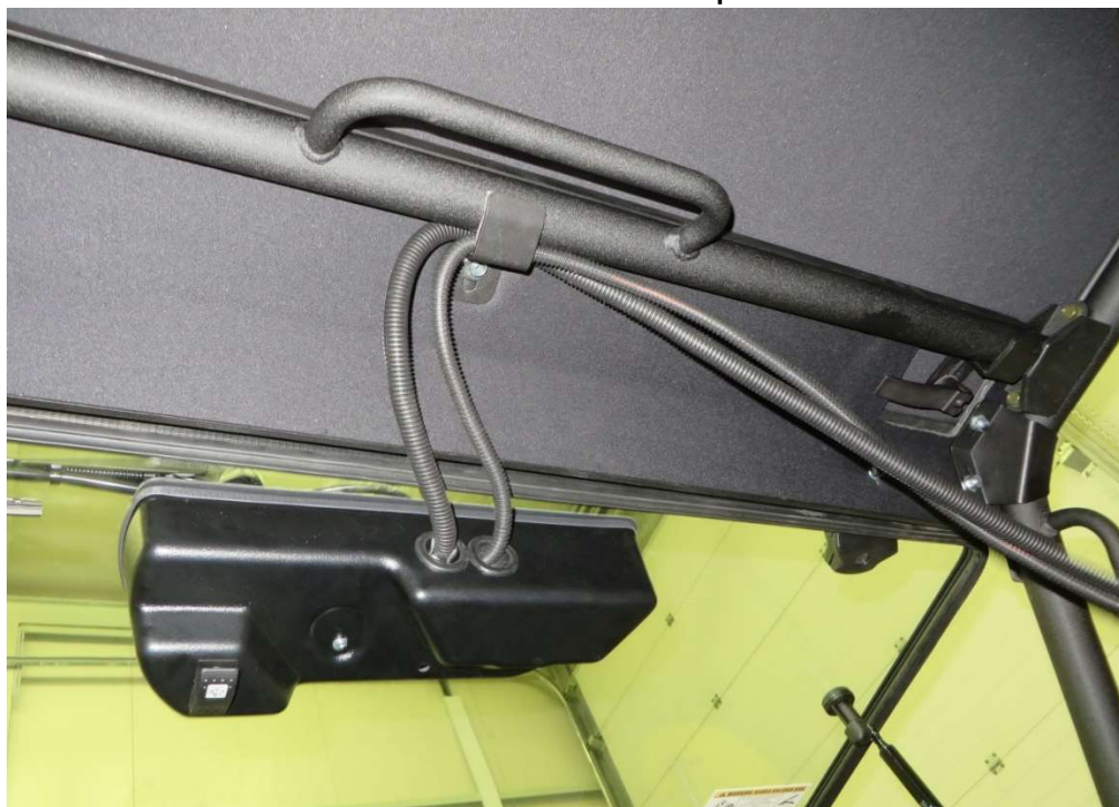
Inside view on installed wiper motor.
