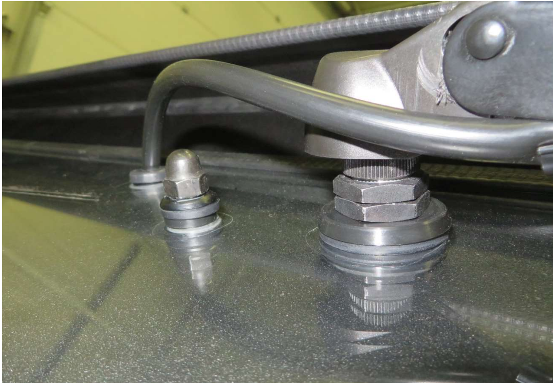
Inside view on installed wiper motor.
