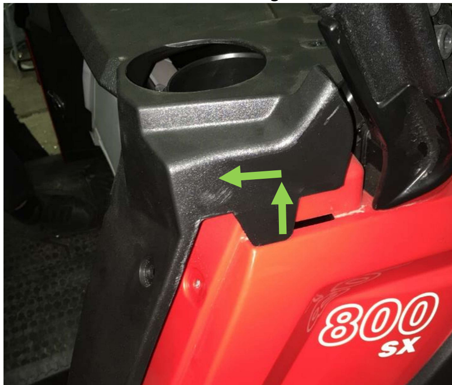
Carefully lift up the dashboard upper cover. Detail view from right side.
