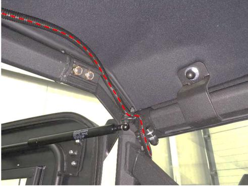
Run the wiper harness from the supply harness to the front wiper motor.
