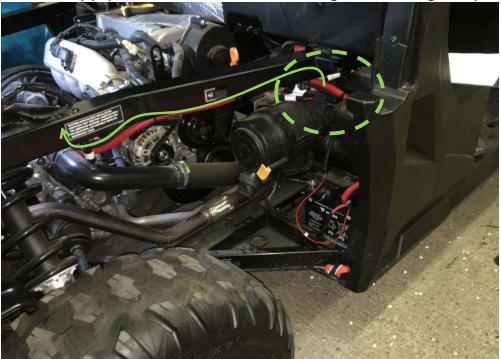
Run the ACC harness brunch from the supply harness to the engine space.
