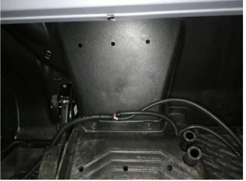
Run the heater harness from the heater to the supply harness. Connect the heater harness with the supply harness.
