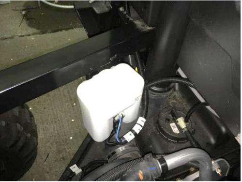
Run the washer harness from the washer tank to the supply harness. Fix the washer harness with the original harness by included tightening straps.
