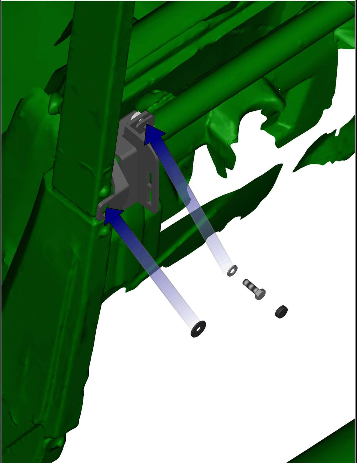
DETAIL VIEW ONTO THE INSTALLED HOLDER BASE FROM INNER SIDE
