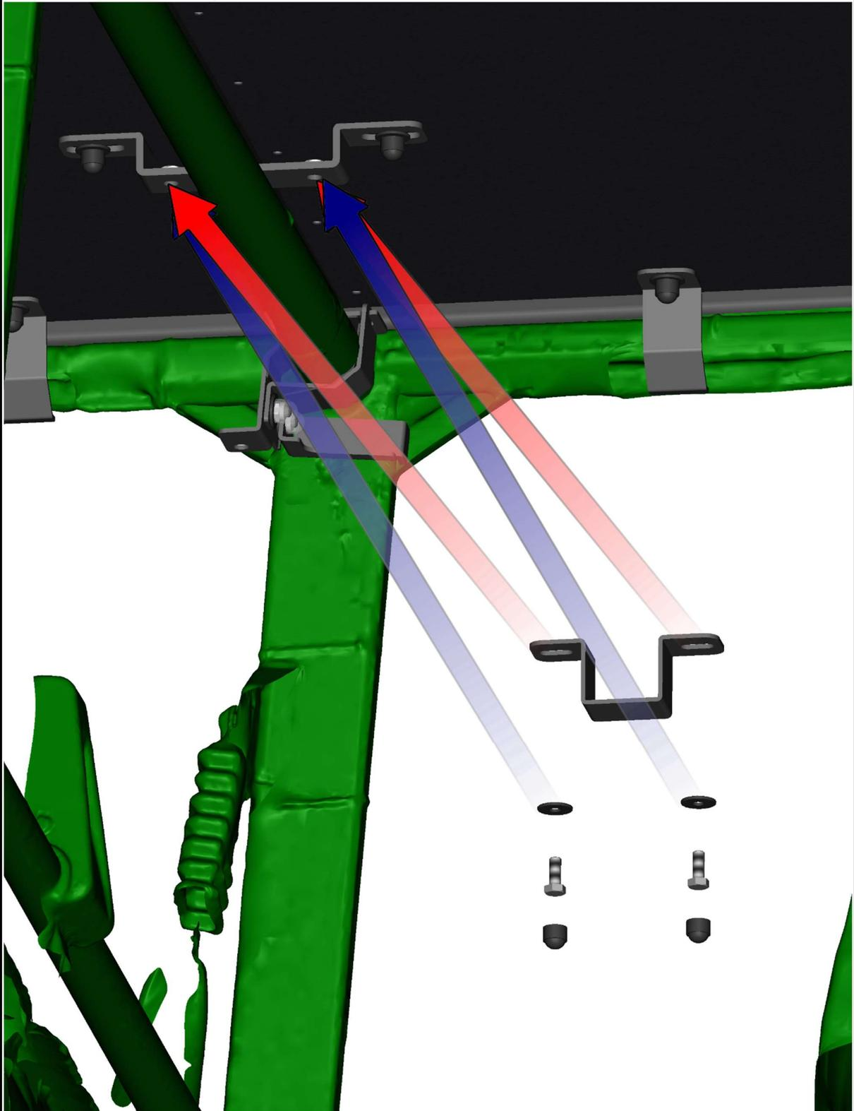
Fix the front roof with the rear roof by included screws, washers, nuts and covers.
