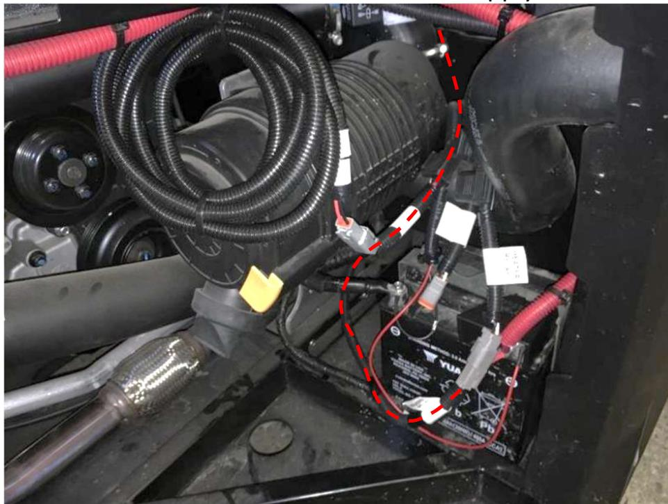
Run the heater hoses through the holes and connect the heater hoses with the heater. Secure heater hoses by included tightening straps.
