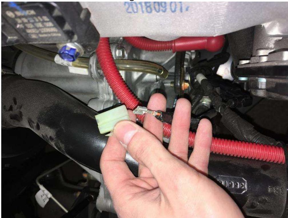
Install the pin from new harness into the same position as the removed pin from previous step.
