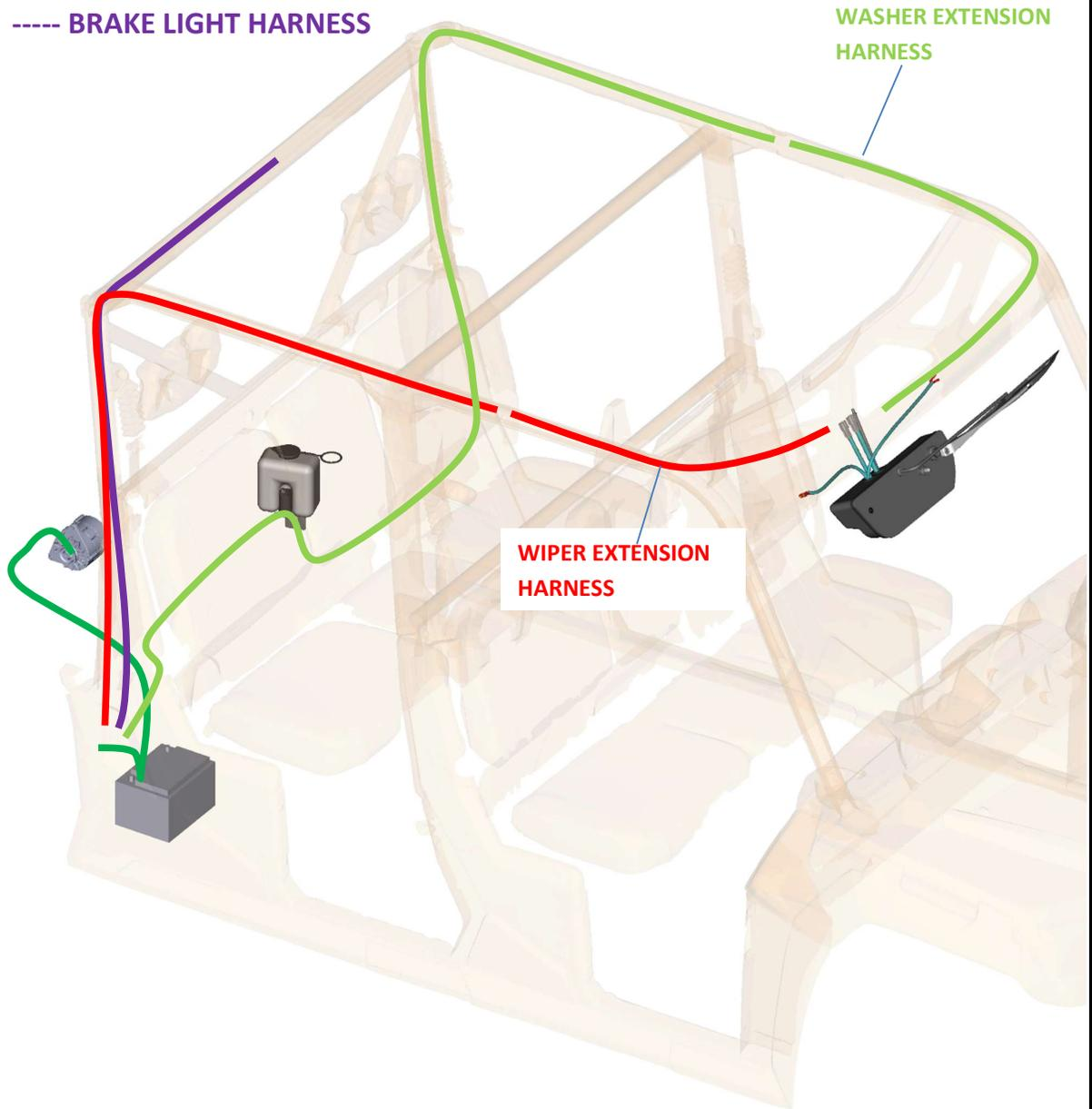
Place the washer harness on the vehicle.
