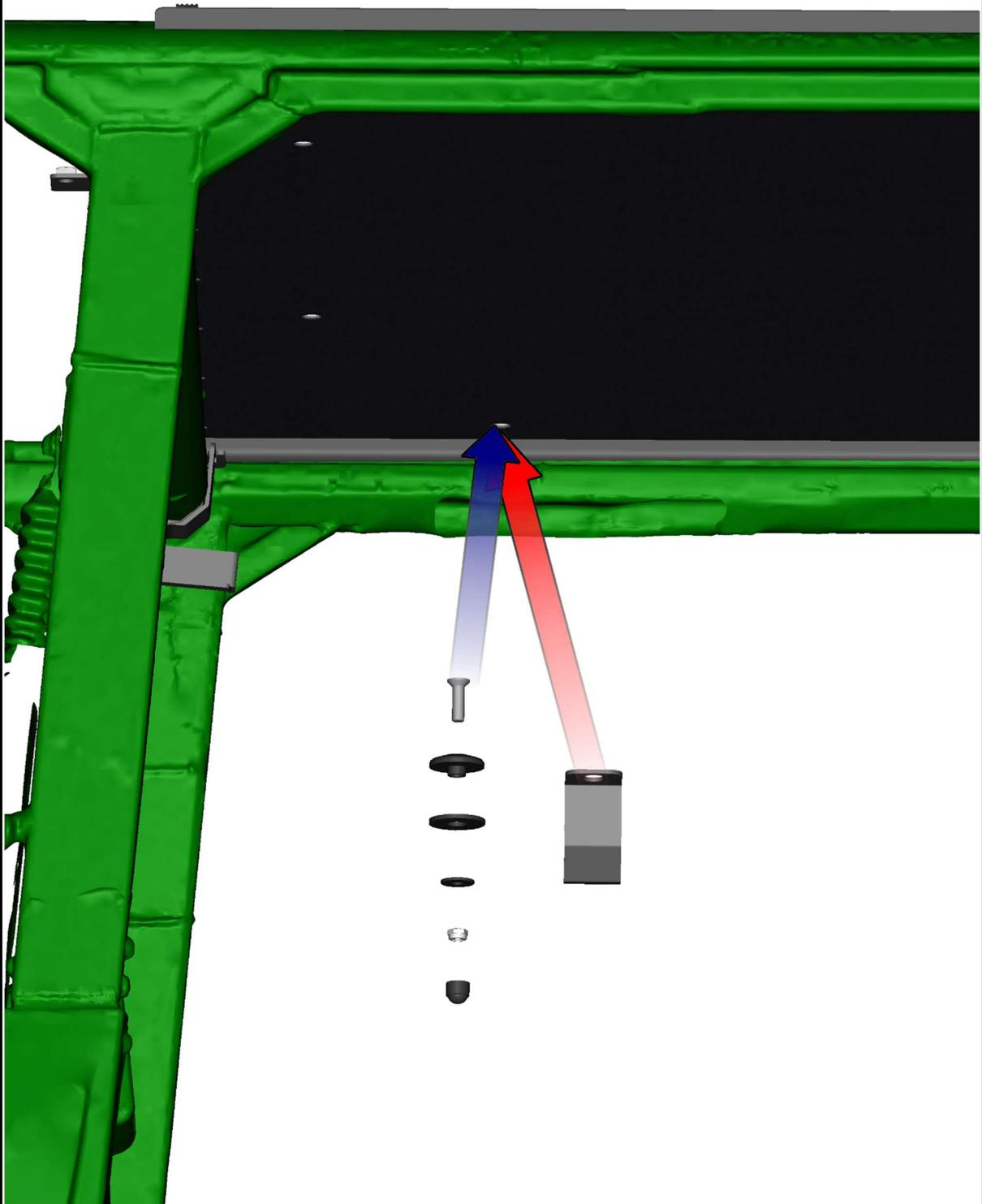
Place the front roof onto the vehicle frame and onto the rear roof.
