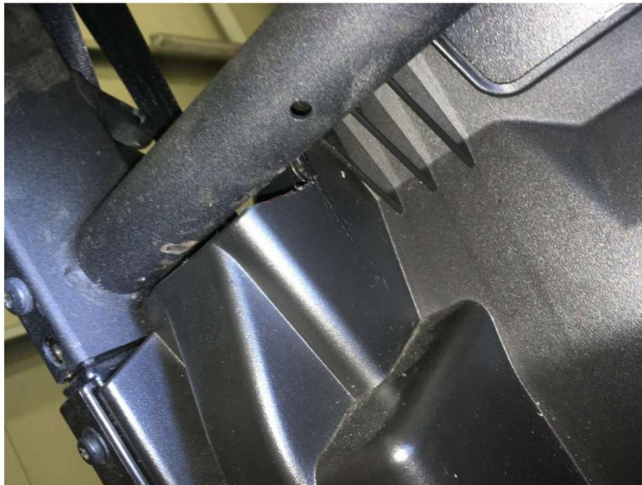
Place the door stop holder base holders onto the vehicle frame.
