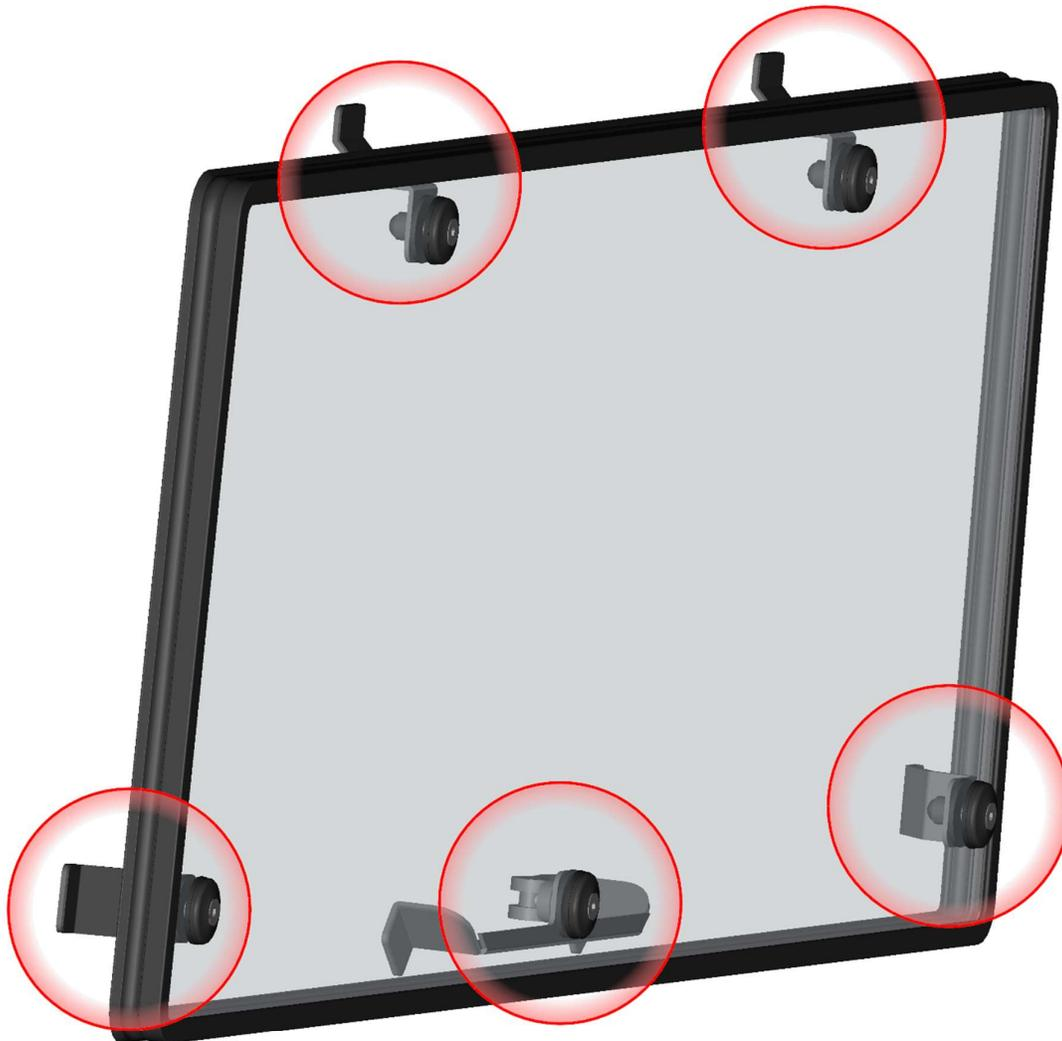
Place the rear window assembly onto the vehicle frame.
