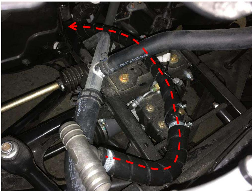
Run the input heater hose (with el. Valve, water pump and **extension hose**) from the rear engine space position to the heater through the central floor tunel.
