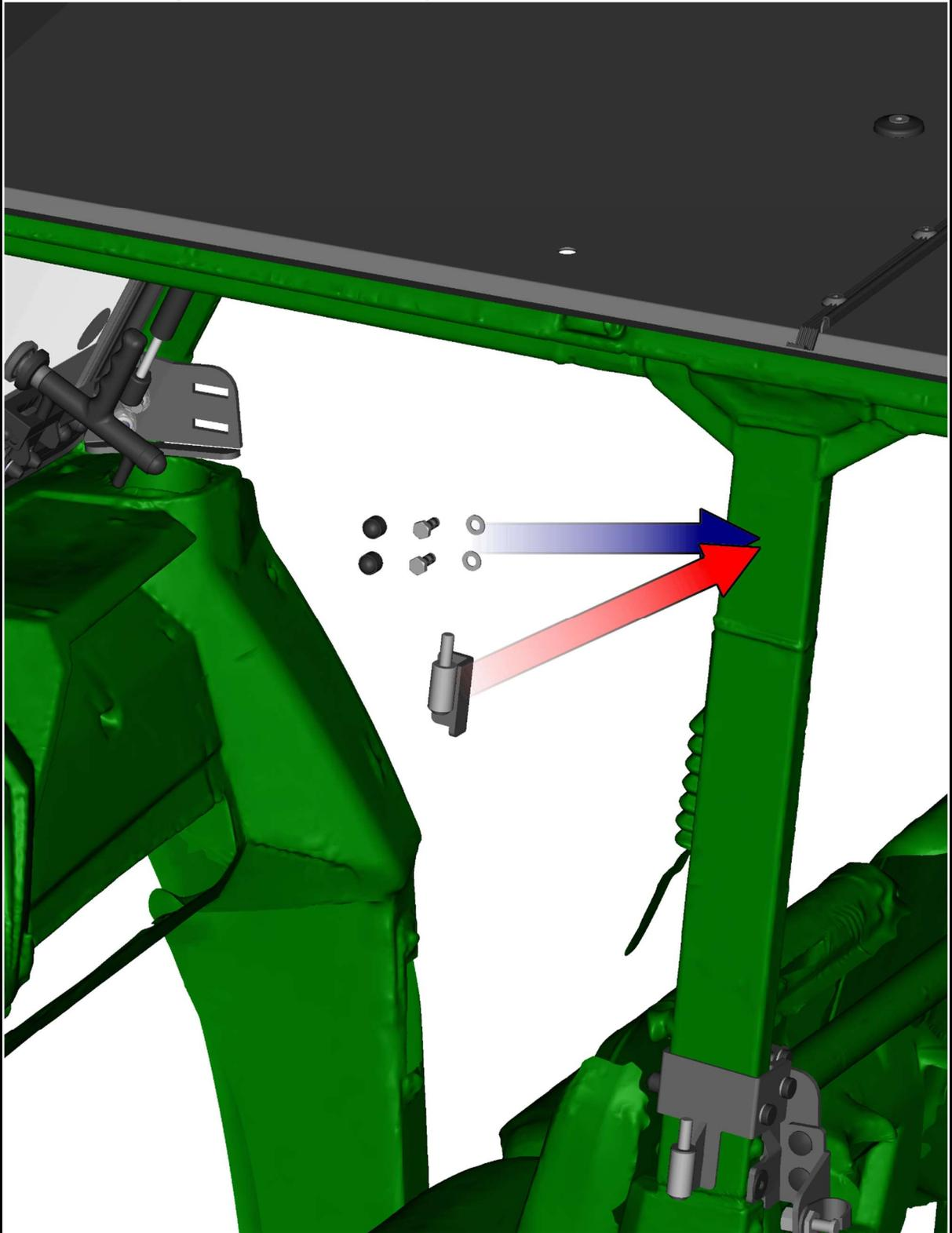
Lubricate the hinges pins and place the door onto the hinges pins.
