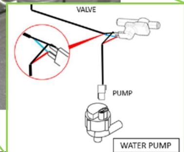
Connect the pump harness with the water pump.
