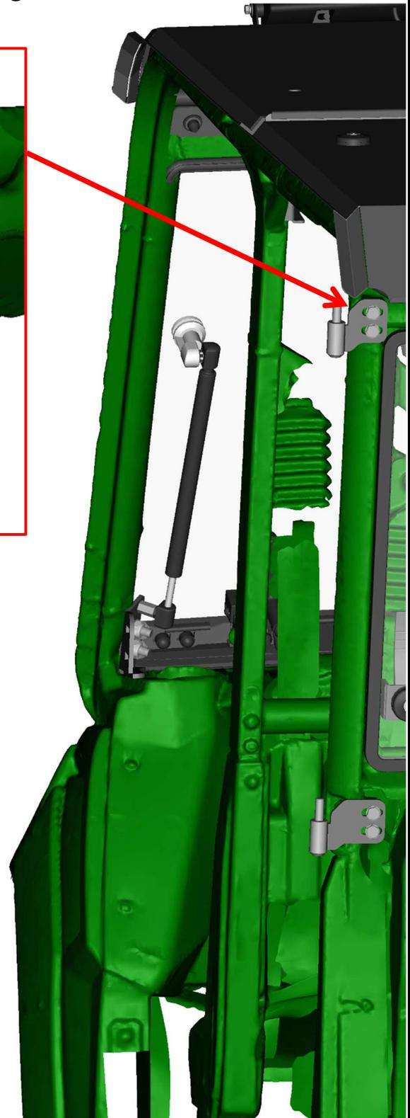
Lubricate the hinges pins and place the door onto the hinges pins.
