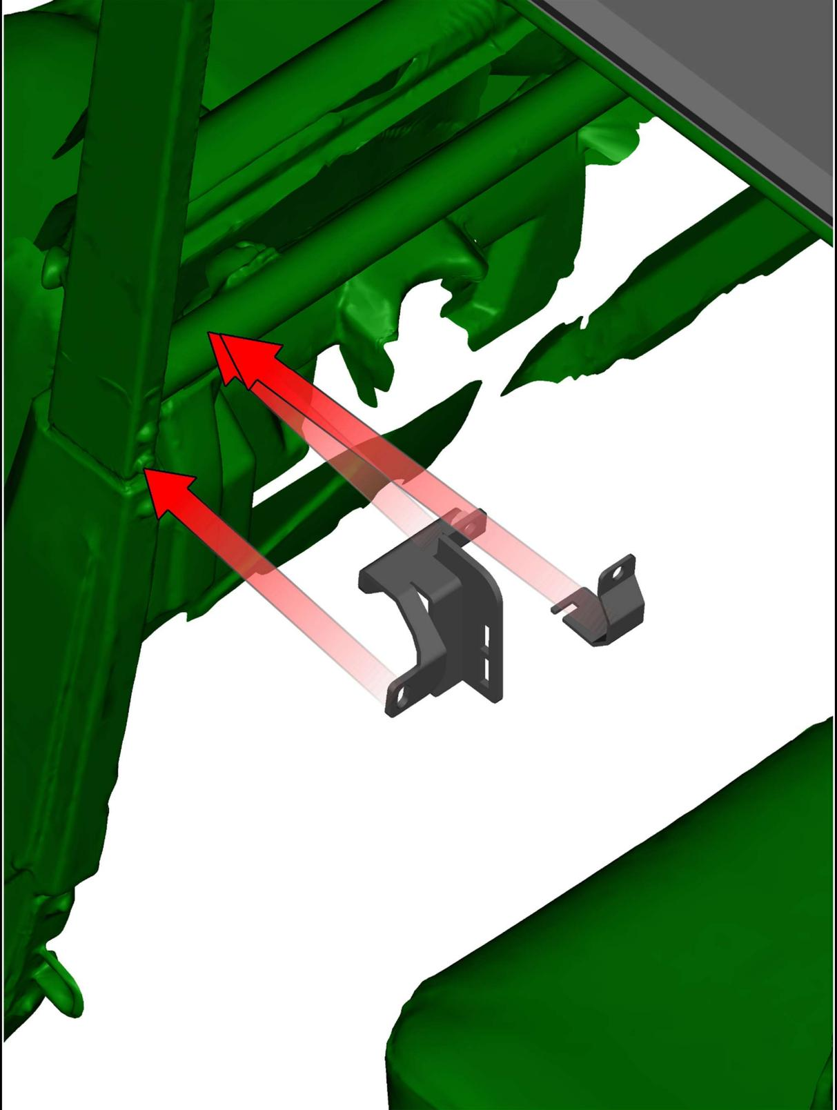
Fix the holder base with the vehicle frame by included washer and original screw. Fix the holder bases by included screw, washer and cover.
