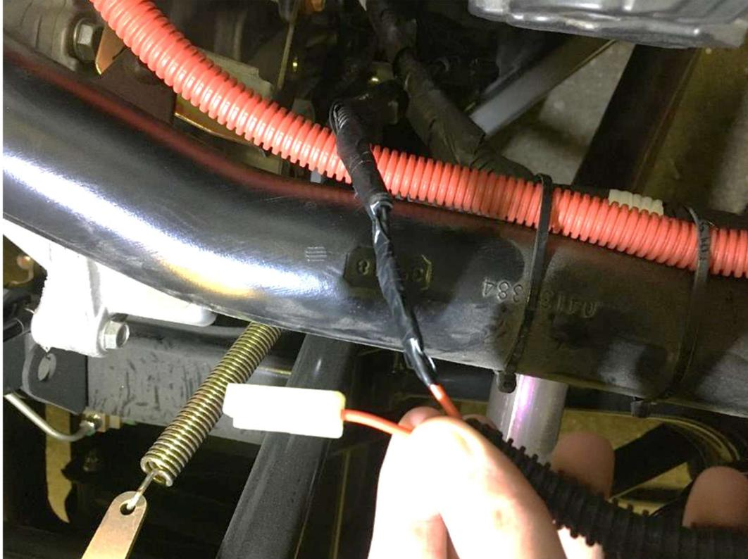
Connect the supply harness with the battery.
