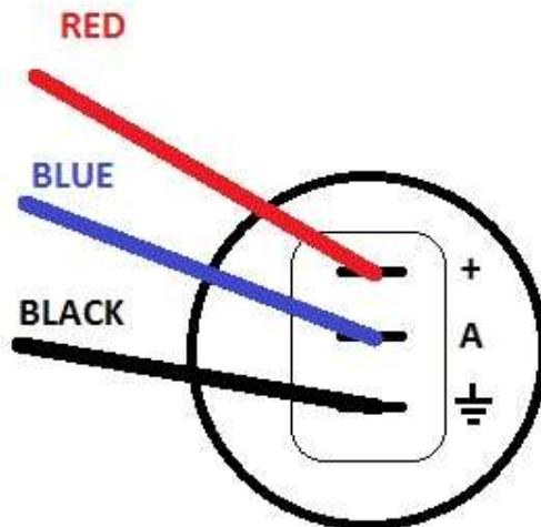
Connect the heater harness with the heater.
