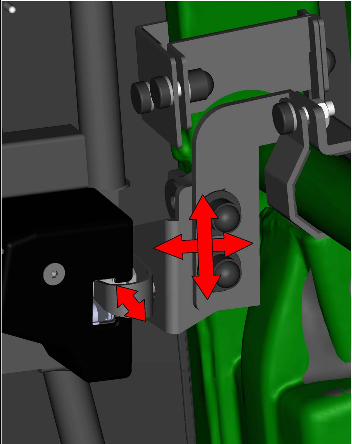
Place the bottom hinge holder onto the hinge base and onto the vehicle frame. Fix the holder with the base by included screw, washers, nut and covers.
