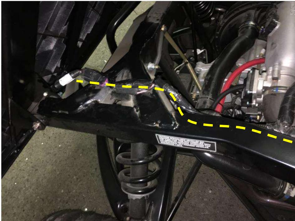
Open the original brake light harness (after the original connection) and connect brake light harness with the original brake light harness **RED/BLUE** wire by included connector. SEE NEXT PAGE
