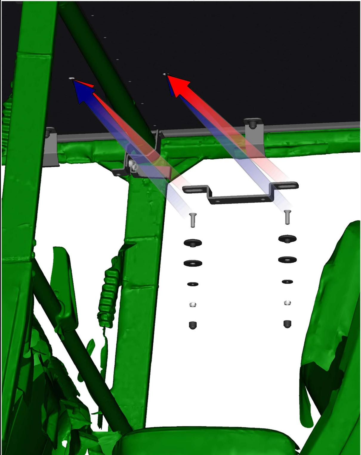
Place the central holder onto the holder base. Fix the holder with the base by included screws, washers, nuts and covers.
