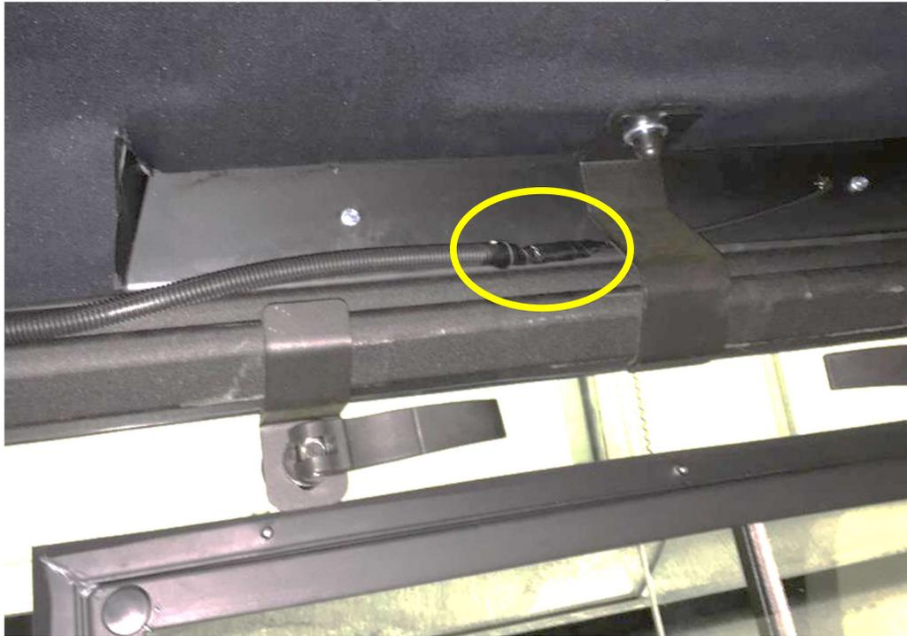
Run the work light harness from the wiper motor assembly to the work light. Connect the work light with the work light harness.
