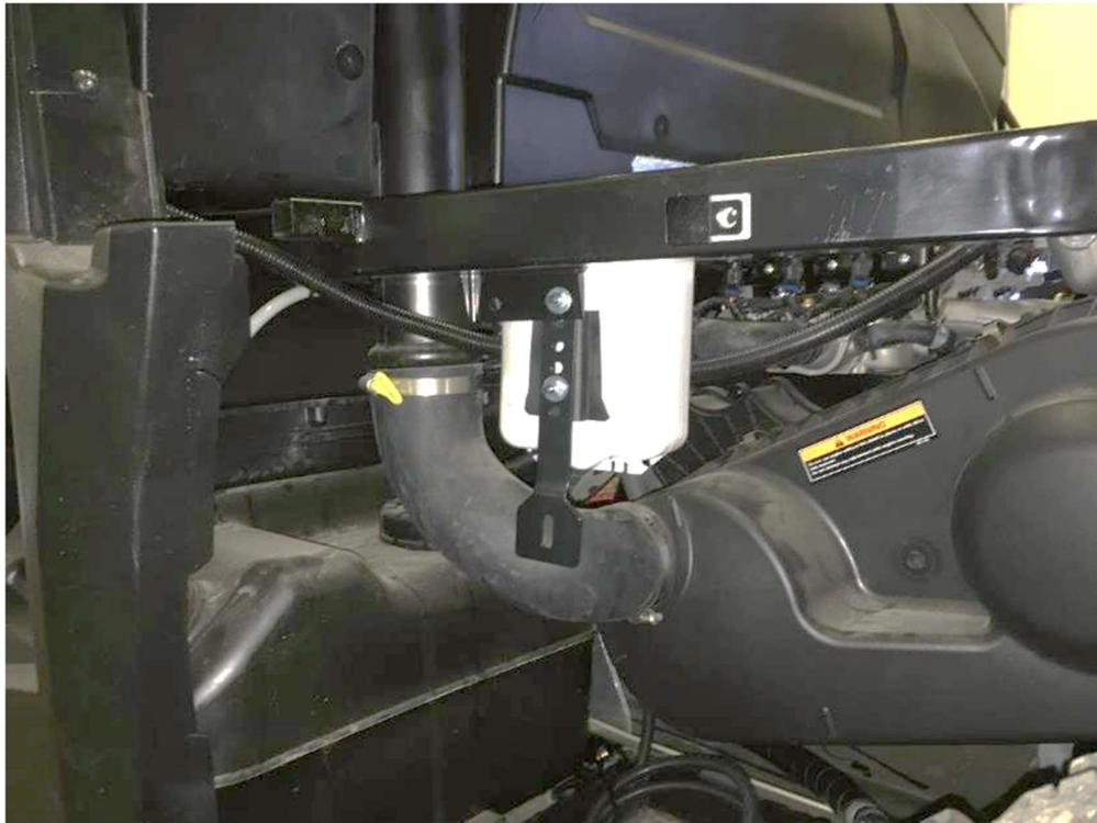
Place the washer tank onto the holder.
