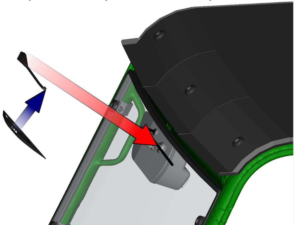
Run the washer harness from the washer tank to the front upper ledge.
