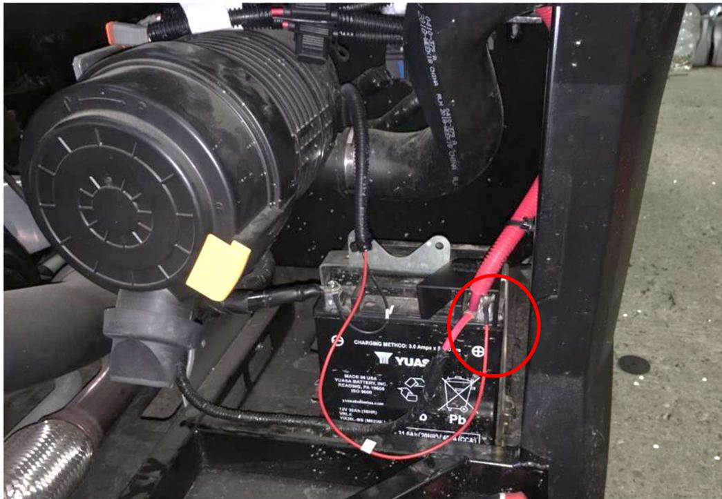
Run the brake light harness from the battery space to the right original brake light.
