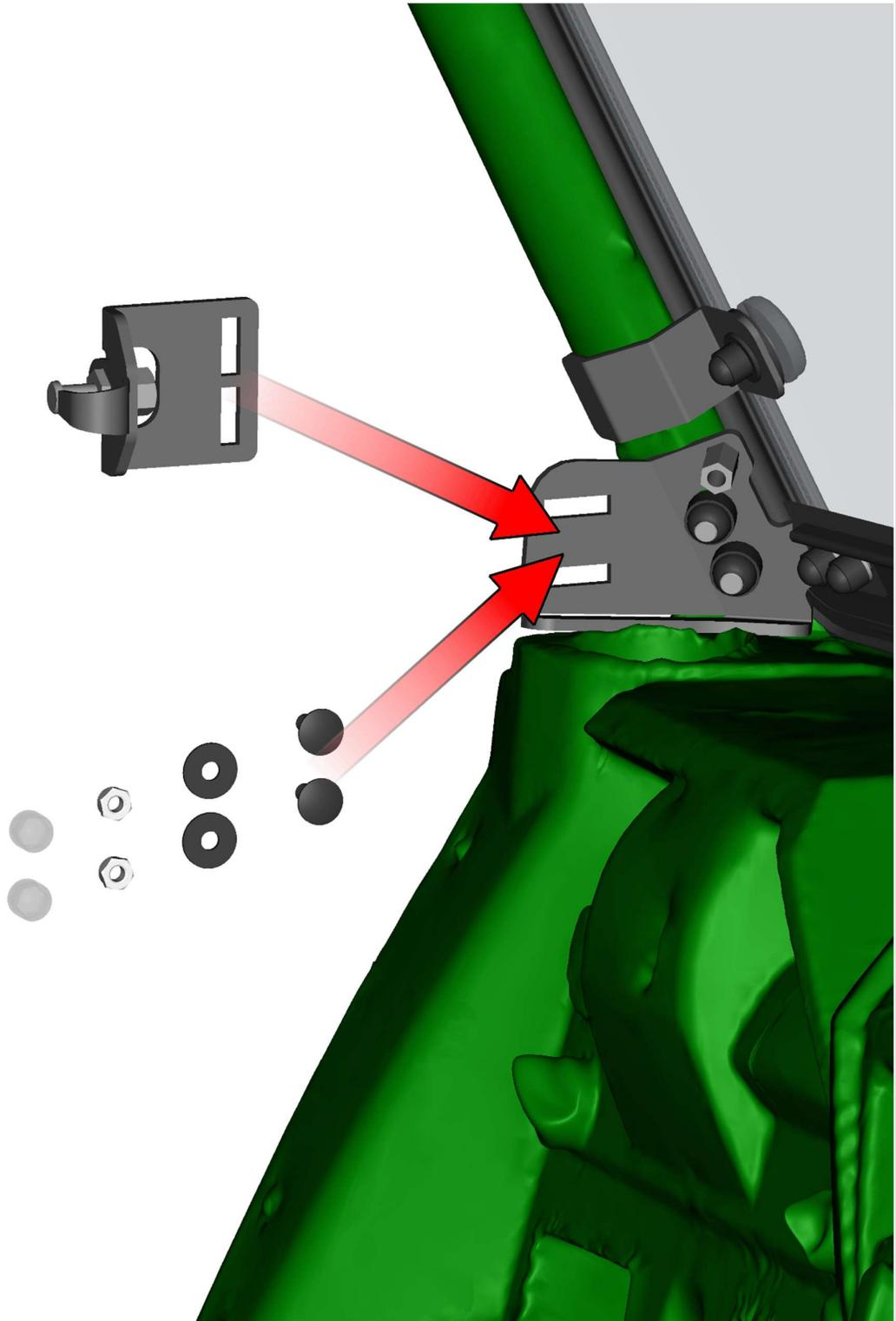
Adjust the door stop assembly to the best position.
