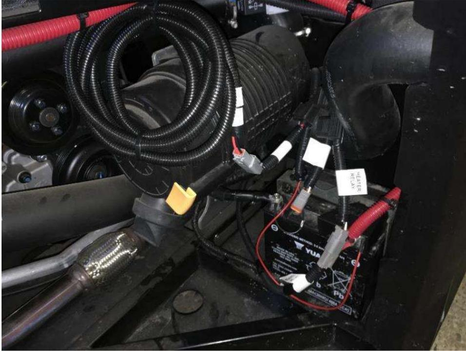
Run the wiper harness from the supply harness to the front wiper motor. 103
