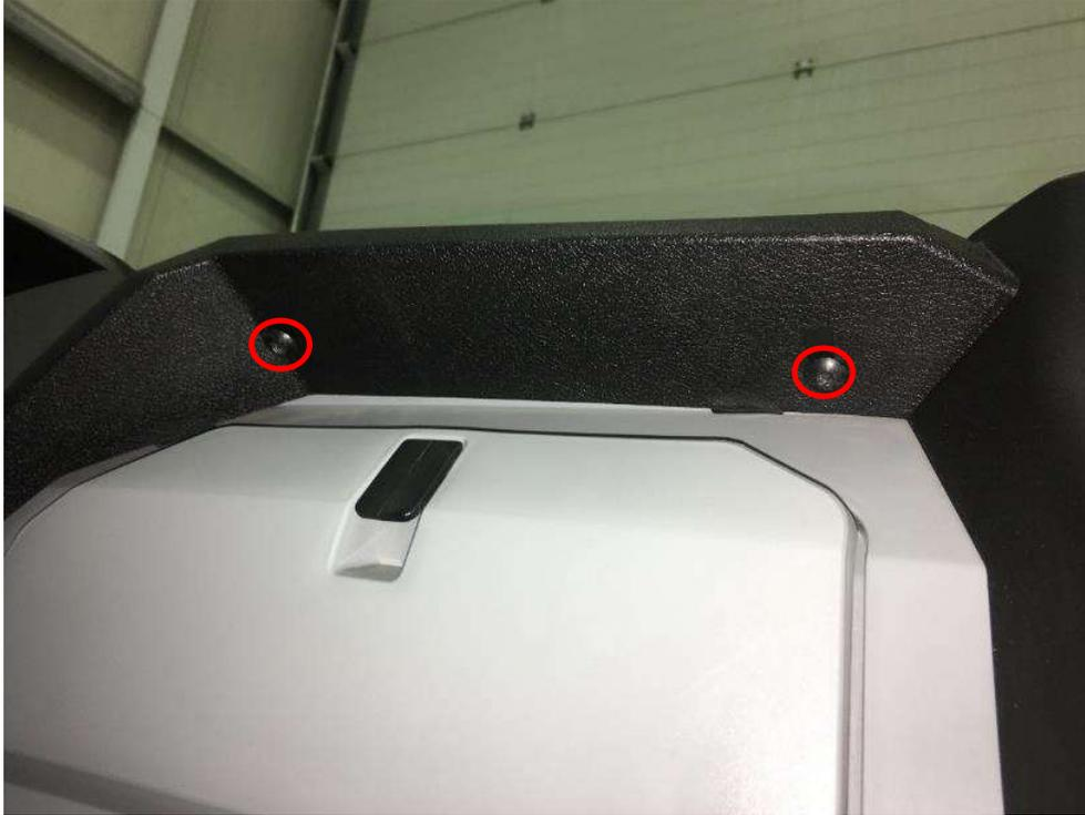
Detail view onto original fixing points.
