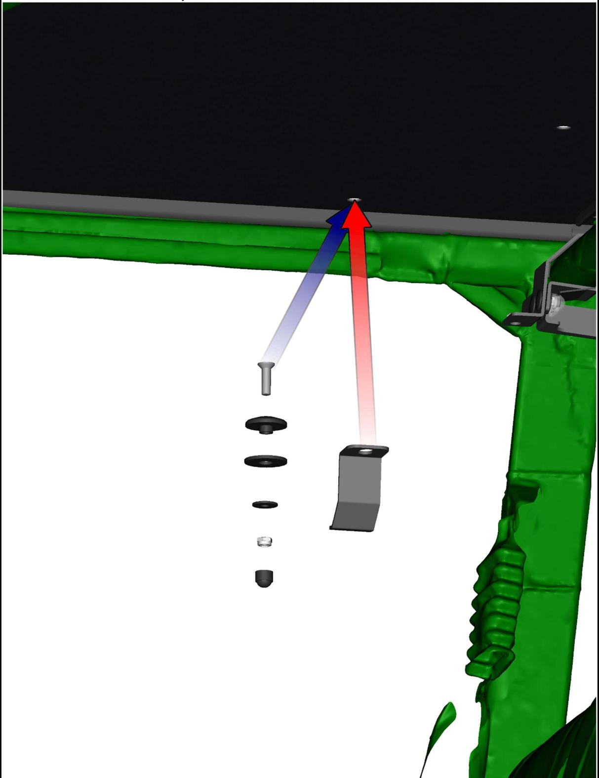
Insert the central holder base between the roof and vehicle frame. Fix the holder base with the front roof and with the rear roof by included screws, washers, nuts and covers. Repeat on the vehicle second side.
