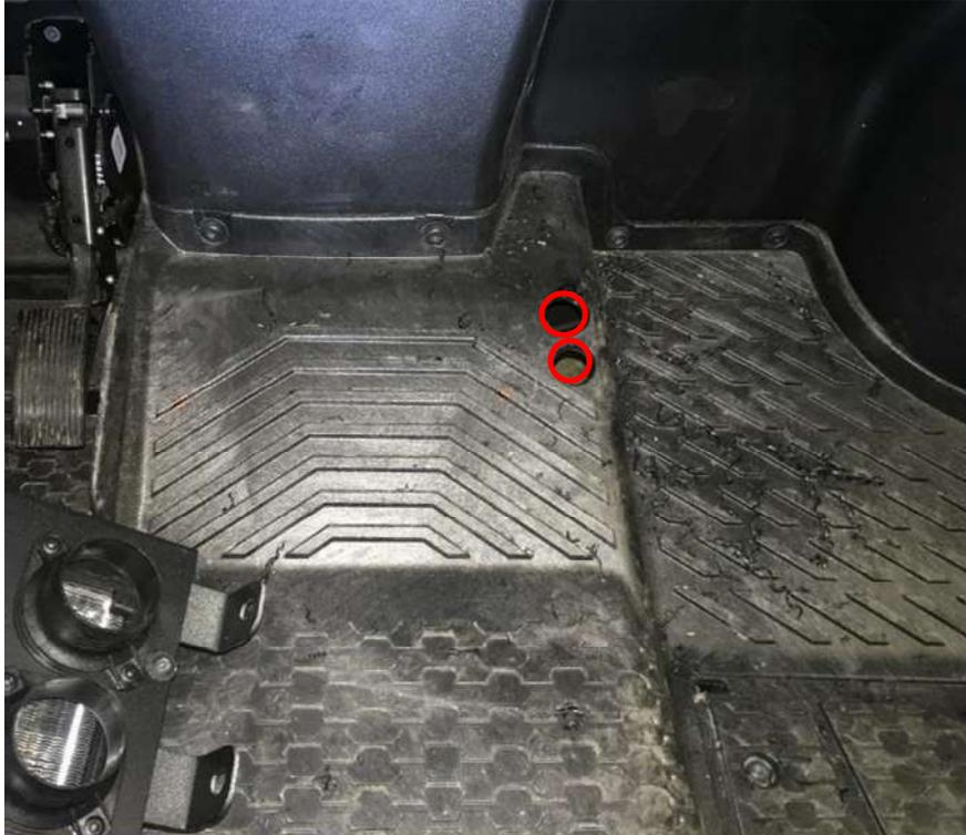
Drill hole  $\varnothing$ 20mm for heater harness.
