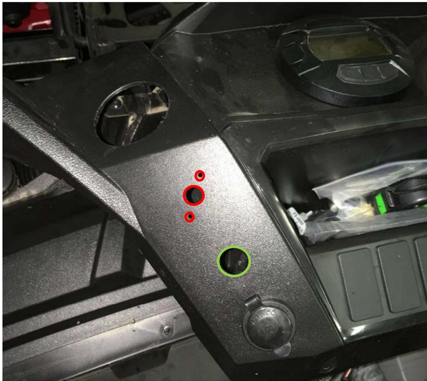
Install switches into the holes.
