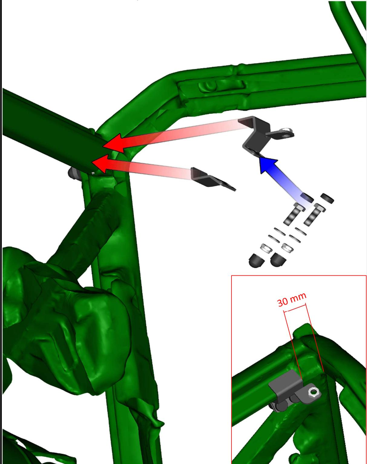
Place the left front gas spring holders onto the vehicle frame. Fix the holders with the frame by included screws, washers, nuts and covers.
