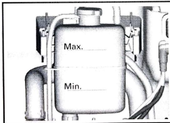
4. Install coolant reservoir cap.
