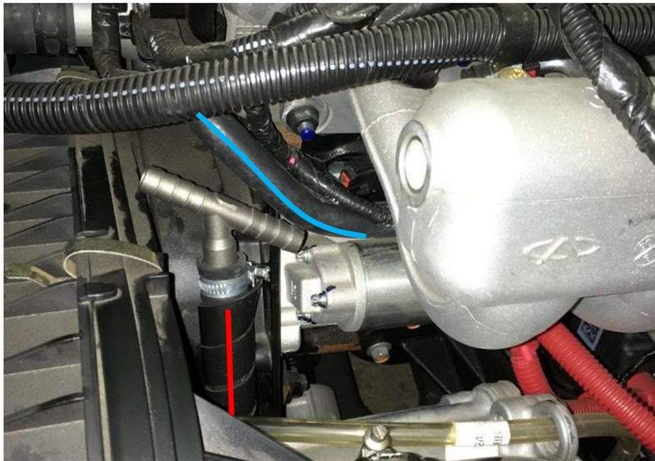
Secure the engine cooling hose by clamps or pliers. Cut the cooling hose between the clamps. Insert the "Y tube" into the cooling hose. Secure the hoses with the coupling by included tightening straps.
