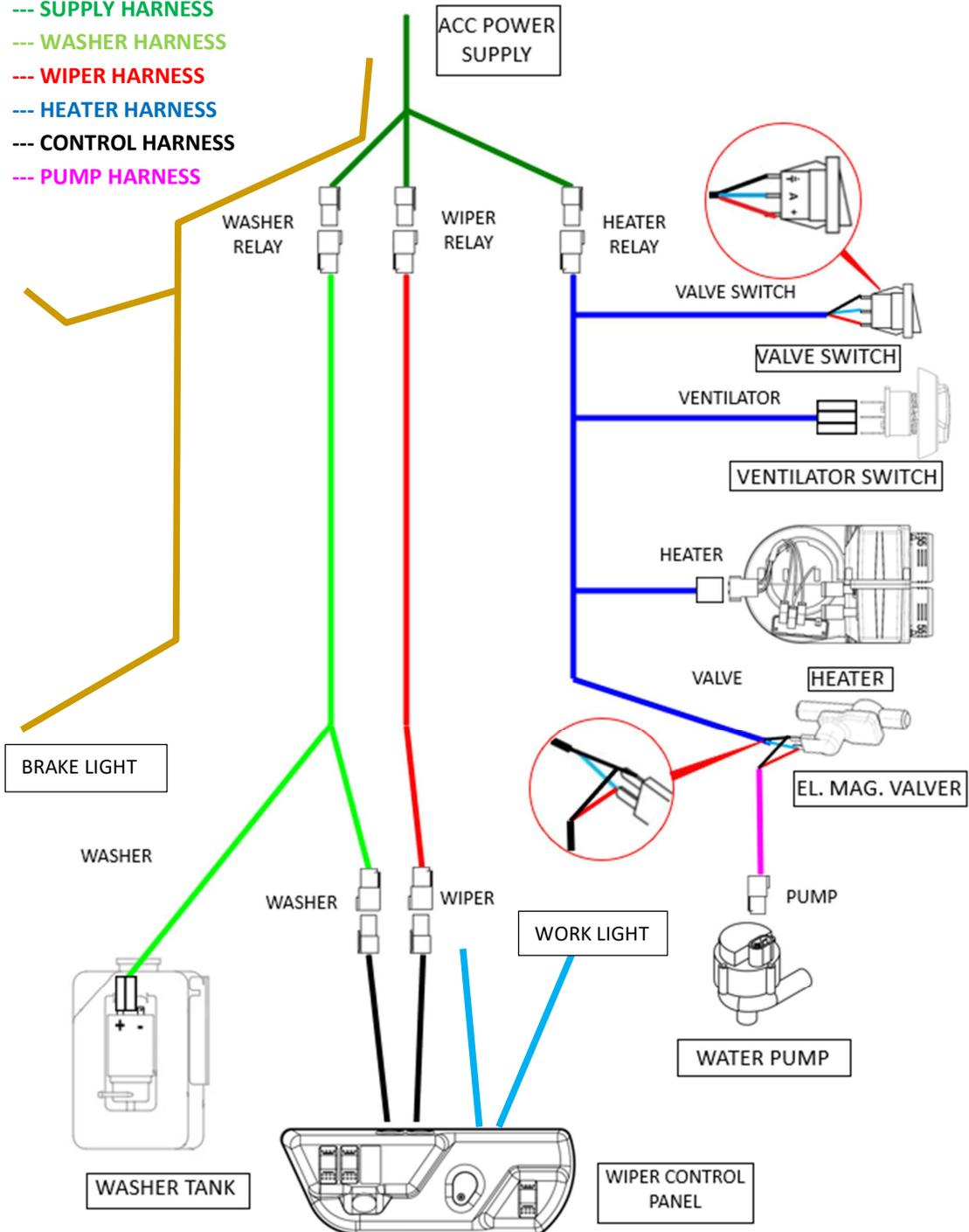
SUPPLY, WIPER AND WASHER HARNESS RUN DIAGRAM
